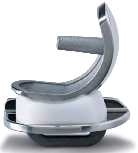
Figure 2. Side View of the Oxford Implant The plastic (polyethylene) insert can float freely on its underlying metal base plate minimizing stress on the cement.
